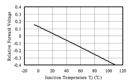
Note :  $\triangle V_F = V_F - V_F (25 \, ^{\circ}\text{C}) = f(Tj); I_F = 2mA$
