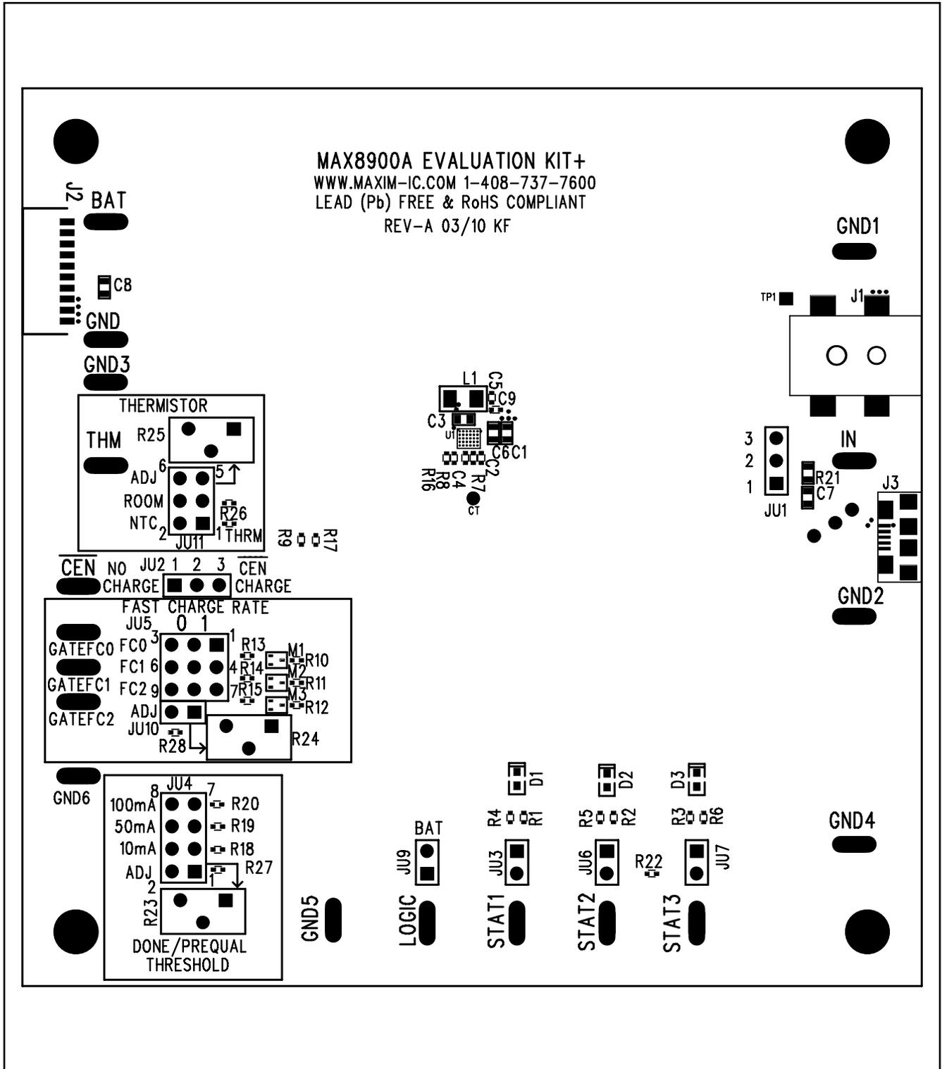
Figure 10. MAX8900A EV Kit Component Placement Guide—Top Layer
