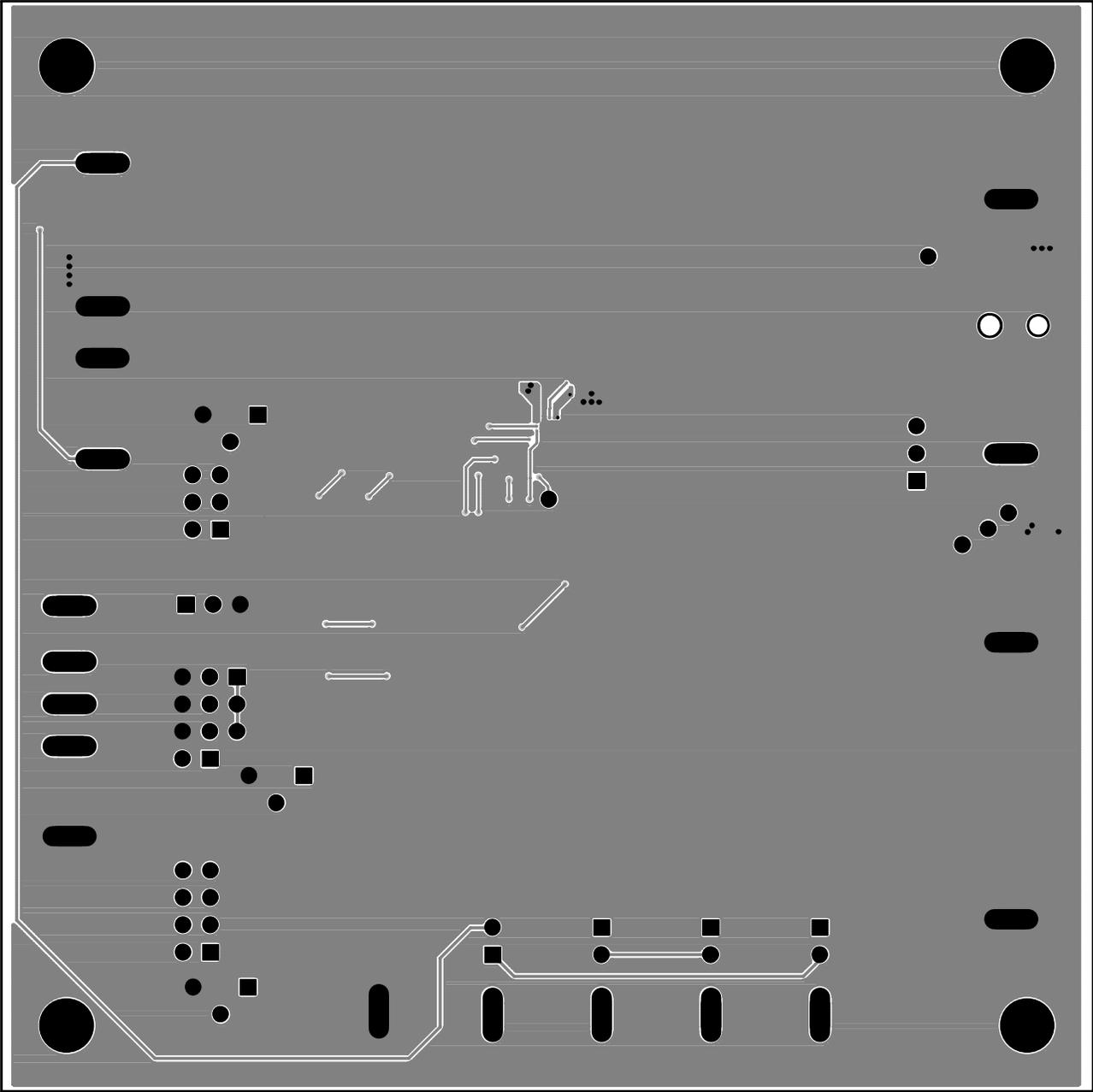
Figure 12. MAX8900A EV Kit PCB Layout—Bottom Layer
