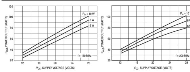
Figure 8. Power Output versus Supply Voltage
