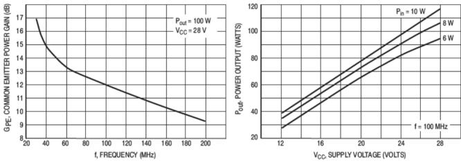
Figure 6. Power Gain versus Frequency
