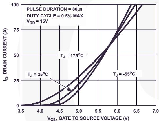
Figure 7. Transfer Characteristics
