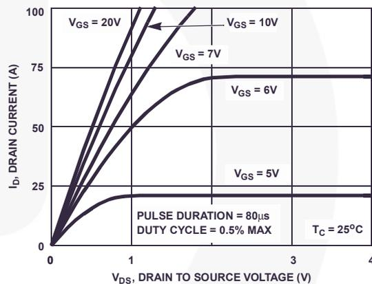
Figure 8. Saturation Characteristics
