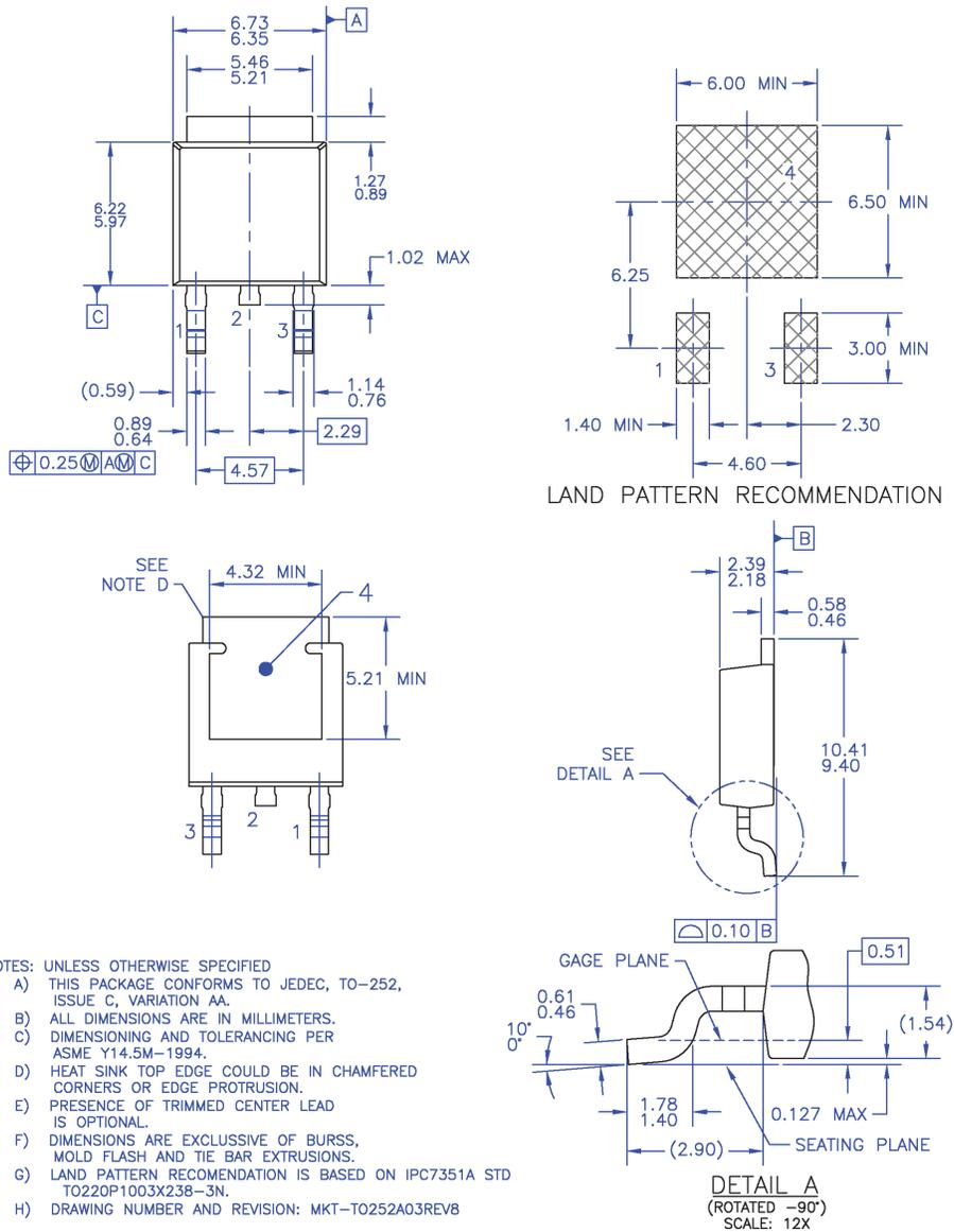
**Figure 21. TO252 (D-PAK), Molded, 3 Lead, Option AA&AB**
