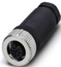
Connector, 5-position, Socket straight M12 SPEEDCON, A-coded, Screw connection, knurl material: Nickel-plated brass, cable gland Pg9, external cable diameter 6 mm ... 8 mm
