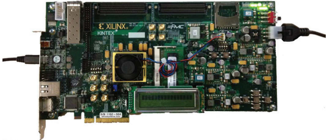
Figure 2-16: Cable Installation for KC705 Board Programming
