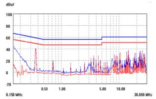
Figure 18. KHHD004A2B Vin+ Line EMC signature using above filter, Vin=48V, Blue=PK, Red=Avq.
