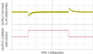
Figure 3. Typical output ripple and noise ( $I_0 = I_{0,max}$ ).
