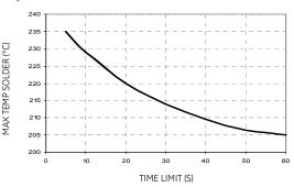
Figure 21. Time Limit, T<sub>lim</sub>, Curve Above 205°C Reflow . Lead Free Soldering
