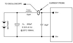
NOTE: Measure input reflected ripple current with a simulated source inductance ( $L_{TEST}$ ) of 12 $\mu$ H. Capacitor  $C_S$  offsets possible battery impedance. Measure current as shown about
