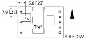
Figure 16. T<sub>ref</sub> Temperature Measurement Location.
