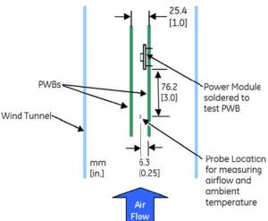
Figure 13. Thermal Test Setup.
