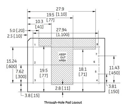
For .025 x .030 rectangular pin, use a .050 diameter plated through hole For .062 diameter pin, use a .076 diameter plated through hole.
