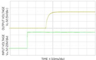
Figure 5.Typical Start-up Using Remote On/Off, negative logic version shown (V  $_{\rm IN}$  = 24V or 48V, Io = I  $_{\rm o,max}$ ).
