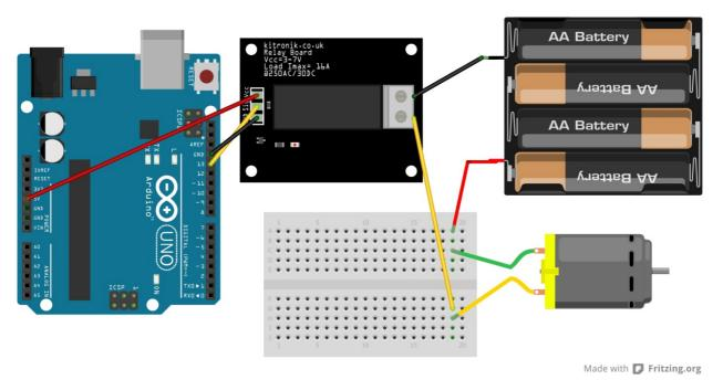
Connect the 5V pin on your Arduino to Vcc. Connect SIG to an output pin on your Arduino. Setting this pin high will trigger the coil switching the load on. Setting this pin low will release the coil and return the relay to its open position. Connect GND to the GND pin on your Arduino.
