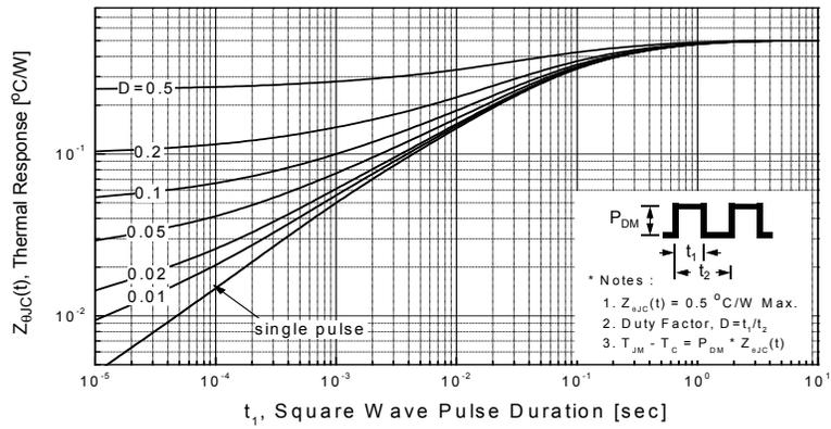
Figure 11-2. Transient Thermal Response Curve - FDPF39N20
