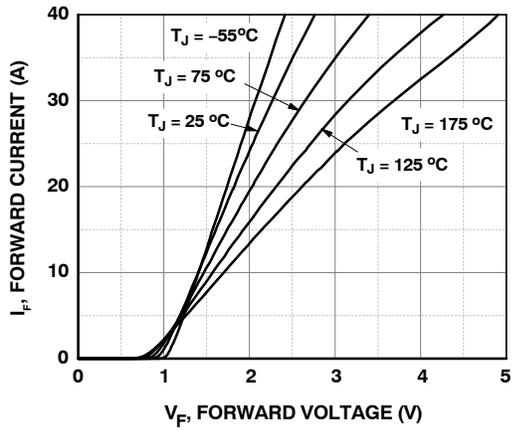
Figure 1. Forward Characteristics
