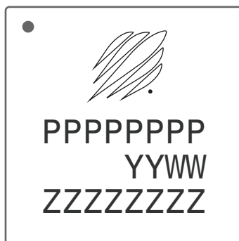
Figure 24 • Package Marking Specifications for PE46130
