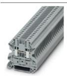
Feed-through terminal block, with partition plate in the bridge shaft, Connection method: Screw connection, Number of positions: 1, Cross section: 0.14 mm² - 6 mm², AWG: 26 - 10, Width: 6.2 mm, Color: gray, Mounting type: NS 35/7,5, NS 35/15
