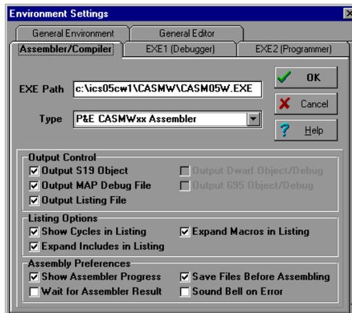
**Figure 1-2. WinIDE Environment Settings Dialog Assembler/Compiler Tab**
