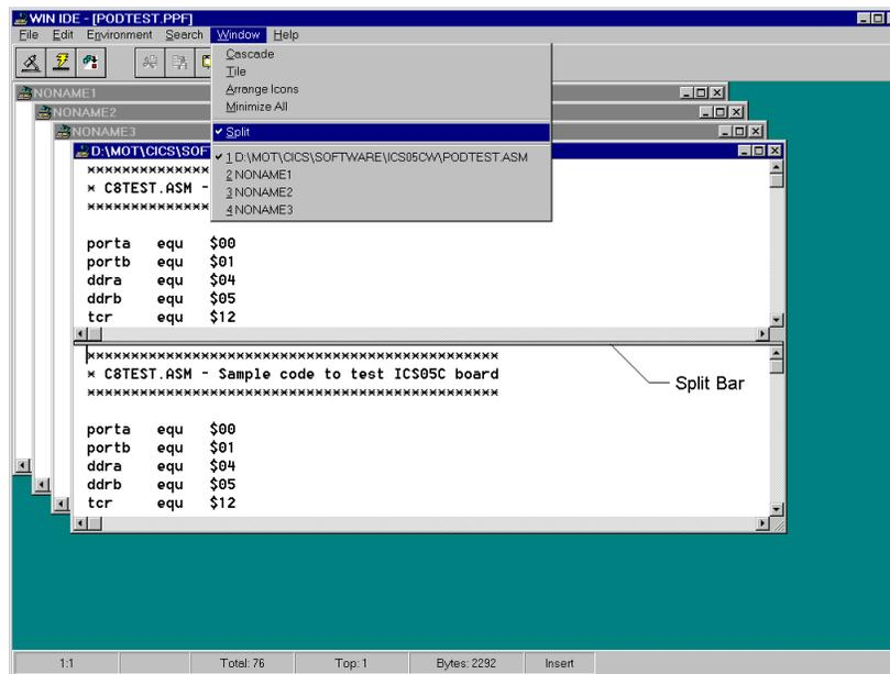
**Figure 4-28. Cascaded Windows with Active Window Split**
