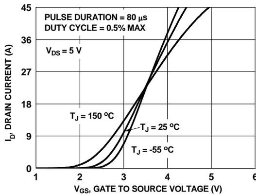
**Figure 5. Transfer Characteristics**
