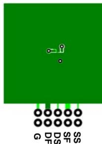
a. 52 °C/W when mounted on a 1 in<sup>2</sup> pad of 2 oz copper.
