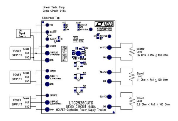
Figure 2. The DC948A connection with Power Supplies, loads, and ON signal source
