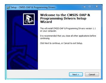
2. During the installation a warning may appear that the publisher cannot be verified depending on Windows security settings. Select, 'install this driver software anyway.' Two drivers are being installed, cmsis-dap and usbdirect. The Windows security window will appear twice, and 'Install this driver software anyway' will need to be selected each time.
