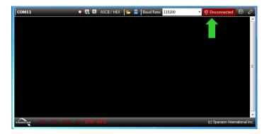
4. Once the terminal is connected, press the space bar on PC keyboard and the welcome message will display. The test application will automatically run the subclock test and report the results. The space bar is used as the input for the USB test.
