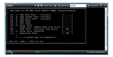
5. To run each of the tests enter the letter next to the test description and follow the prompts. For example: p <enter> will test the potentiometer (R11). The application will prompt the user for a sequence of rotations of the potentiometer, and report the test result.
