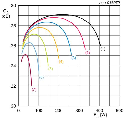
$I_{Dq} = 100 \text{ mA}$ ;  $f = 108 \text{ MHz}$ ;  $t_p = 100 \text{ }\mu\text{s}$ ;  $\delta = 20 \text{ \%}$ .
