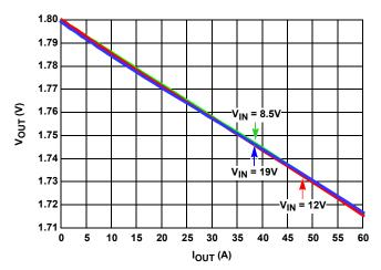
FIGURE 1. LOAD LINE REGULATION
