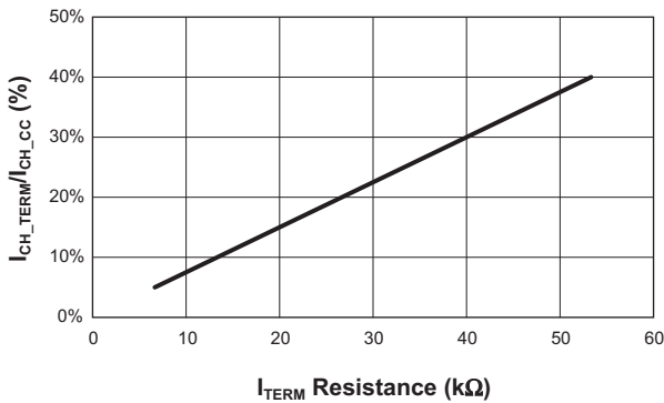
Termination Current to Constant Current Ratio (%) vs. Termination Resistance
