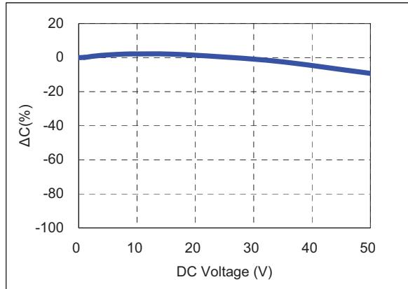
4) Bias TCC characteristics (Agilent 4284A, 1kHz, 1Vrms, 25Vdc)
