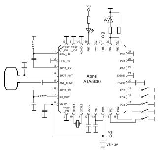
Figure 2. ATA5830N Flash Application Schematic
