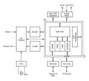
Figure 1. ATA5830N Block Diagram
