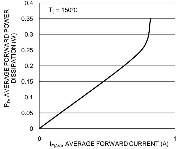
Figure 2. Forward Power Dissipation
