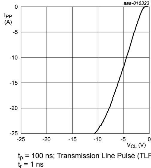
**Fig. 10. Dynamic resistance with negative clamping; typical values**
