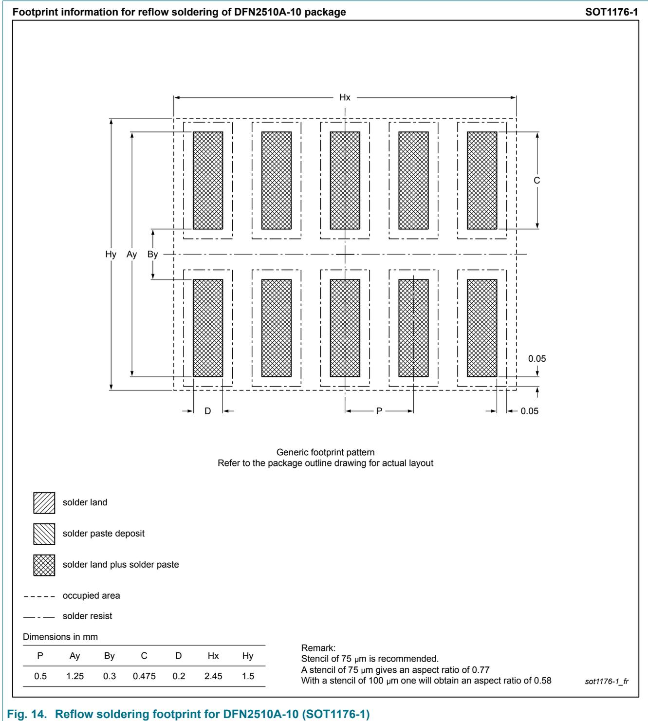
Fig. 14. Reflow soldering footprint for DFN2510A-10 (SOT1176-1)
