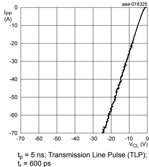
**Fig. 12. Dynamic resistance with negative clamping; typical values**
