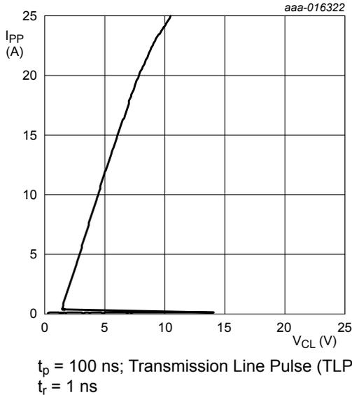
**Fig. 9. Dynamic resistance with positive clamping; typical values**
