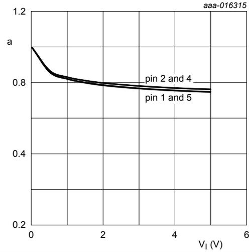
$$a = \frac{C_{line}}{C_{line}(V_I = 0 V)}$$
