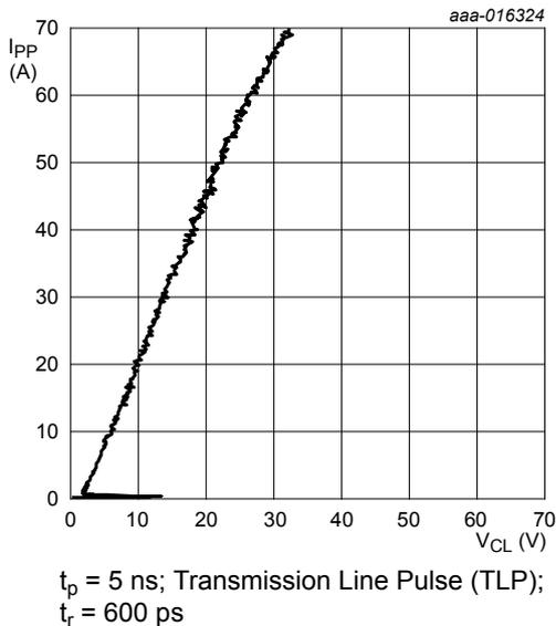
**Fig. 11. Dynamic resistance with positive clamping; typical values**
