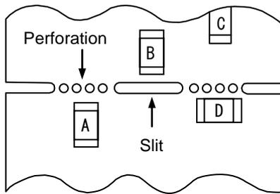
\*1 A > D is valid when stress is added vertically to the perforation as with Hand Separation.
