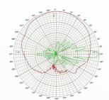
Typical azimuth and elevation pattern SA24-90-17-WB
