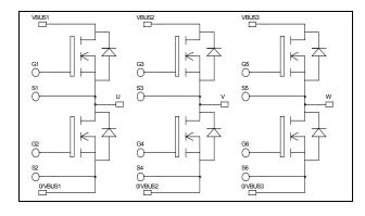
$$\begin{split} V_{DSS} &= 1000 V \\ R_{DSon} &= 350 m \Omega \text{ typ } \text{ } \text{ } \text{ } \text{Tj} = 25^{\circ} \text{C} \\ I_D &= 22 \text{A} \text{ } \text{ } \text{ } \text{C} = 25^{\circ} \text{C} \end{split}$$
