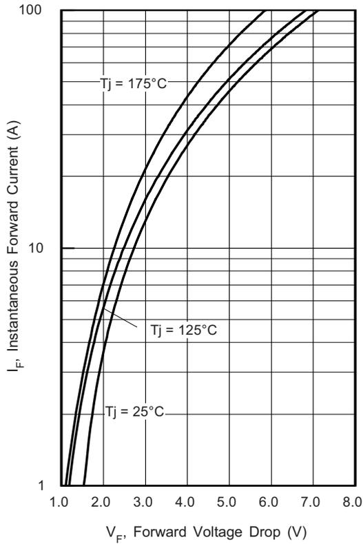
Fig. 1 - Typical Forward Voltage Drop vs. Instantaneous Forward Current
