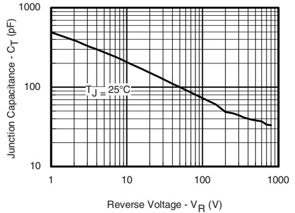
Fig. 3 - Typical Junction Capacitance vs. Reverse Voltage
