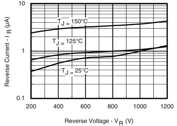
Fig. 2 - Typical Reverse Current vs. Reverse Voltage
