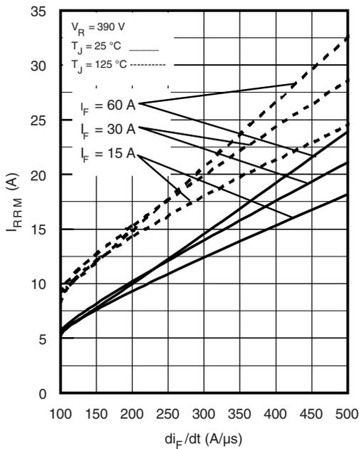
Fig. 6 - Typical Recovery Current vs.  $di_F/dt$  (Per Leg)
