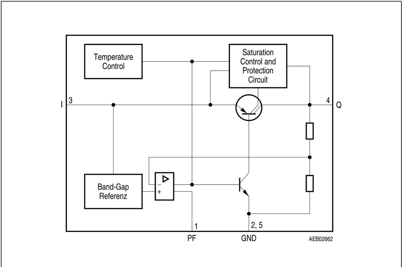
**Figure 2**      **Block Diagram**
