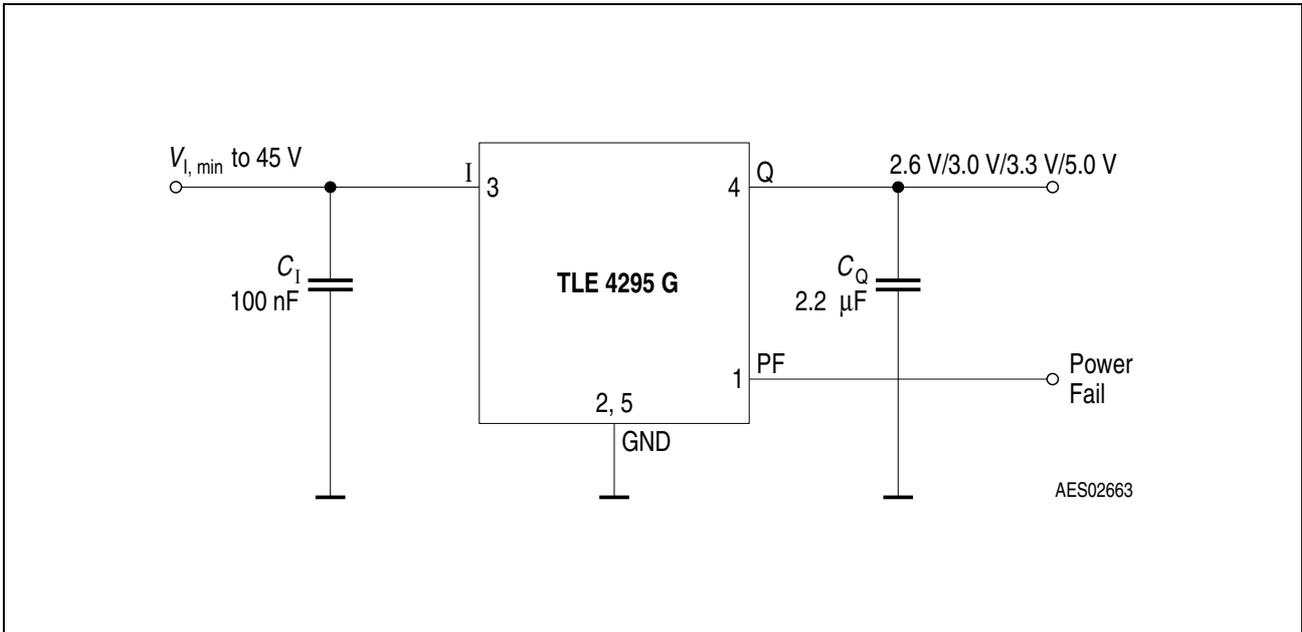
**Figure 3 Application Circuit**
