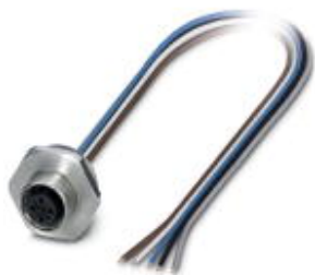
Sensor/actuator flush-type socket, 4-pos., M12, A-coded, front/screw mounting with M20 x 1.5 thread, with 0.5 m TPE litz wire, 4 x 0.34 mm 2 , brass version
