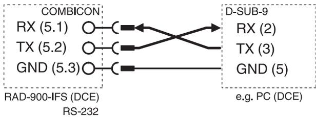
Figure 8 RS-232 interface pin assignment (DCE - DTE)
