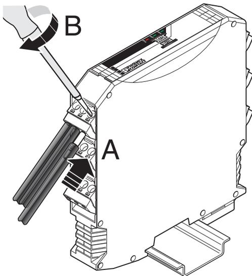
Figure 6 Connecting the cables
