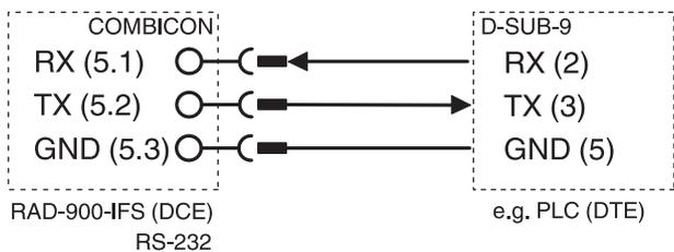
Figure 9 RS-232 interface pin assignment (DTE - DCE)
