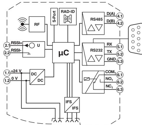
Figure 2 Circuit diagram
