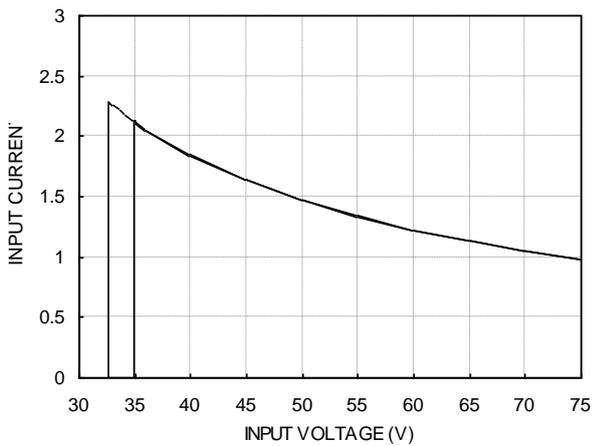
**Figure 3:** full load input characteristics at room temperature.
