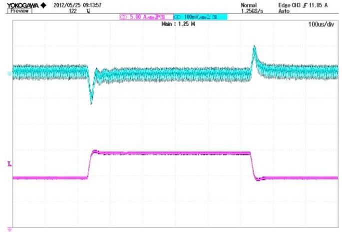
**Figure 9:** Output voltage response to step-change in load current (50%-75%-50% of full load;  $di/dt = 2.5A/\mu s$ ). Load cap:  $10\mu F$ , tantalum capacitor and  $1\mu F$  ceramic capacitor. Top Trace:  $V_{out}$ ;  $100mV/div$ ; Bottom Trace: output current:  $5A/div$ , Time:  $100\mu s/div$
