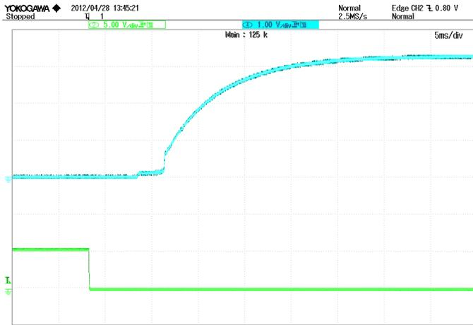
**Figure 4:** Turn-on transient at zero load current (5ms/div).
