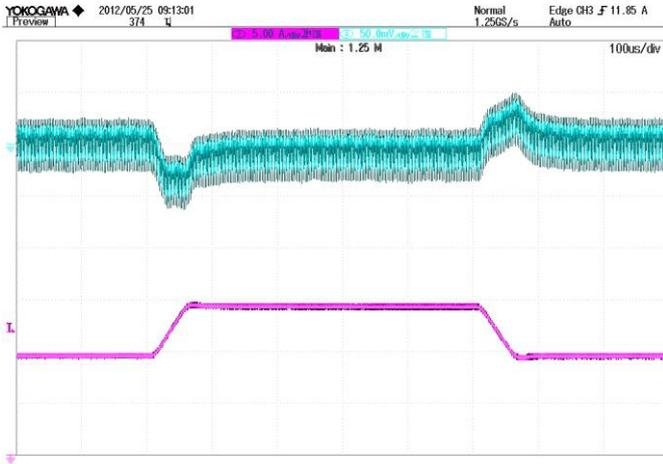
**Figure 8:** Output voltage response to step-change in load current (50%-75%-50% of full load;  $di/dt = 0.1A/\mu s$ ). Load cap:  $10\mu F$ , tantalum capacitor and  $1\mu F$  ceramic capacitor. Top Trace:  $V_{out}$ ;  $50mV/div$ ; Bottom Trace: output current:  $5A/div$ , Time:  $100\mu s/div$
