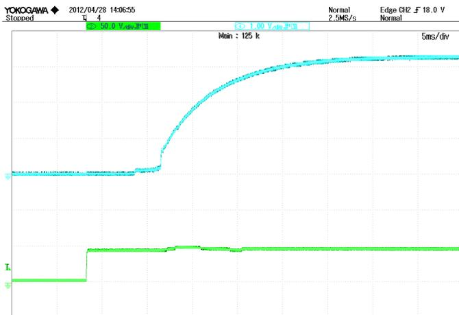
**Figure 6:** Turn-on transient at zero load current (5 ms/div).
