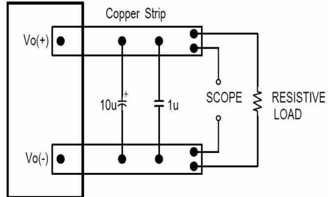
**Figure 13:** Output voltage noise and ripple measurement test setup.
