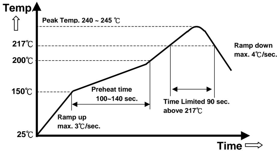
Note: The temperature refers to the pin of V48SC, measured on the +Vout pin joint.
