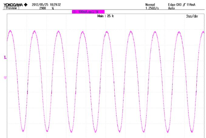
**Figure 11:** Input Terminal Ripple Current,  $i_c$ , at max output current and nominal input voltage with  $12\mu H$  source impedance and  $33\mu F$  electrolytic capacitor ( $100mA/div$ ,  $2\mu s/div$ ).
