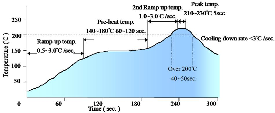
Note: The temperature refers to the pin of V48SC, measured on the +Vout pin joint.
