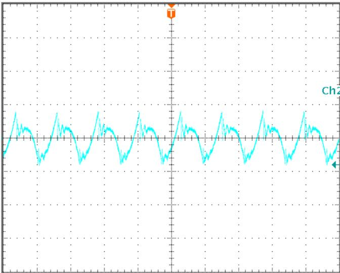
**Figure 14:** Output voltage ripple at nominal input voltage and max load current (20 mV/div, 2 us/div)
