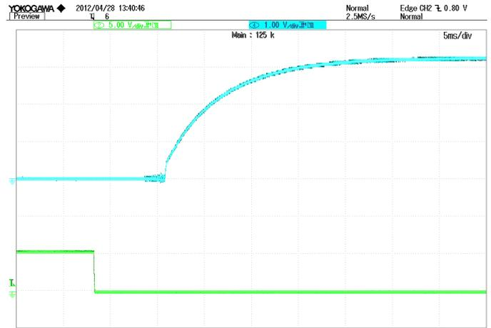
**Figure 5:** Turn-on transient at full load current (5ms/div).
