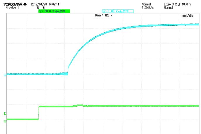
**Figure 7:** Turn-on transient at full load current (5 ms/div).
