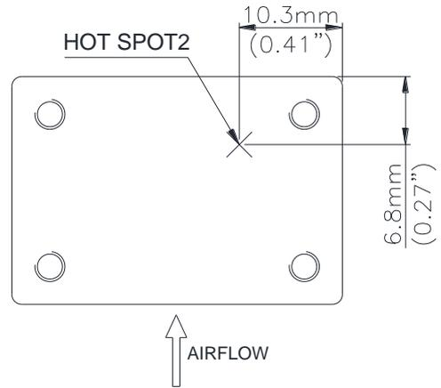
**Figure 20:** \* Hot spot 2 temperature measured point. The allowed maximum hot spot 2 temperature is defined at 110°C
