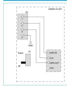
**Terminal design:** Signalling push-in terminal block (X51 COM) 1 DATA IN
