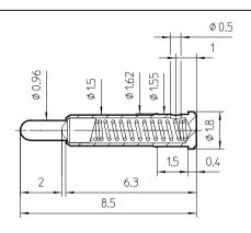
Note: Contact P/N is for basic contact, please add suffix for plating code and, for socket contacts, assembly code.
