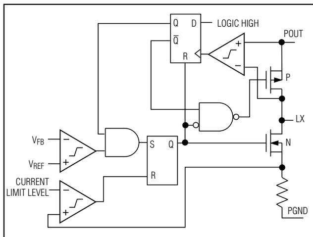
Figure 5. Controller Block Diagram in PFM Mode
