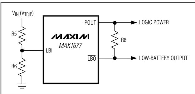
Figure 6. Setting the Low-Battery Trip Threshold
