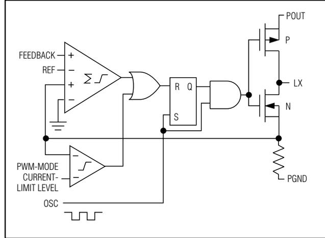
Figure 4. Controller Block Diagram in PWM Mode
