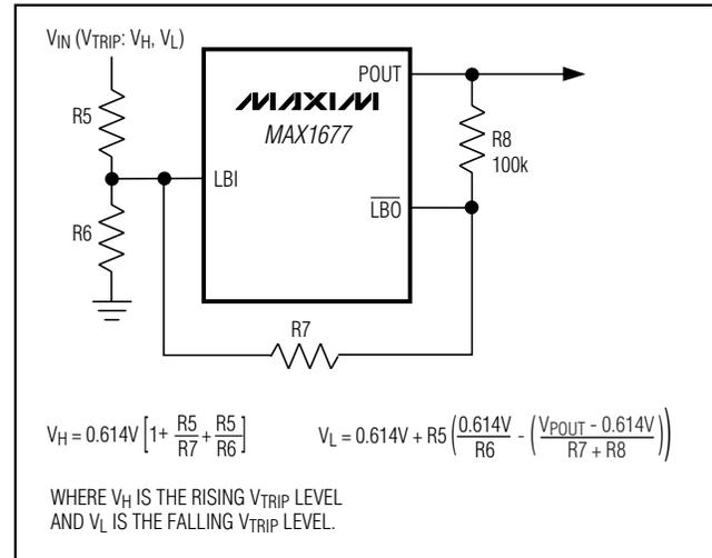
Figure 7. Adding External Hysteresis to the LBI Comparator
