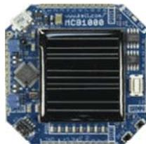
The Keil MCB1343 Evaluation Board introduces the new LPC134x family of ARM Cortex-M3 processor-based devices, allowing you to create and test working programs for this advanced architecture. The MCB1343 has a wide range of interfaces making it a great starting point for your next Cortex-M3 project.
