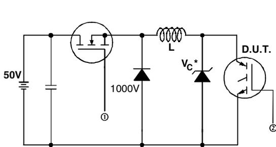
\* Driver same type as D.U.T.;  $V_c = 80\%$  of  $V_{ce(max)}$
