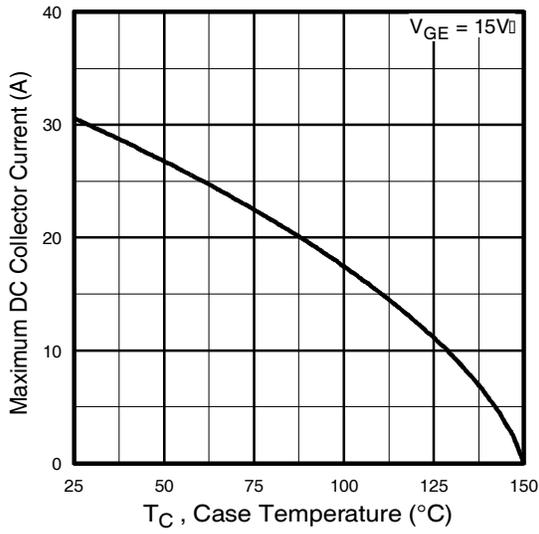
**Fig. 4 - Maximum Collector Current vs. Case Temperature**
