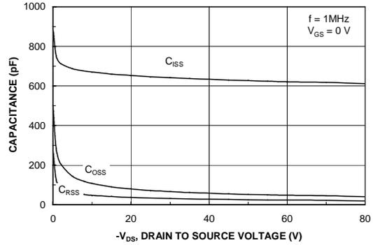
Figure 8. Capacitance Characteristics.
