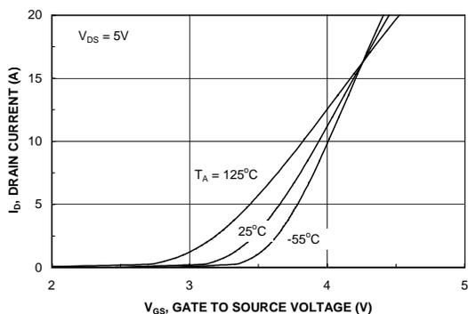
Figure 5. Transfer Characteristics.
