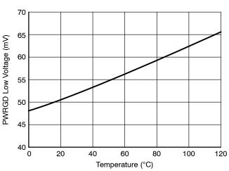
Figure 14. PWRGD Output Low Voltage vs. Temperature
