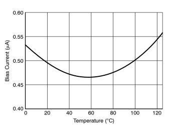
Figure 8. V<sub>FB</sub> Bias Current vs. Temperature
