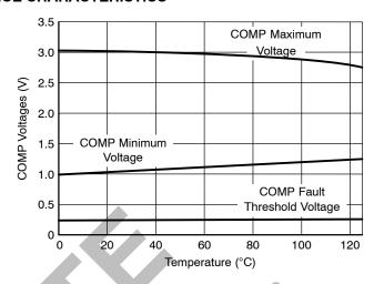
Figure 10. COMP Voltages vs. Temperature
