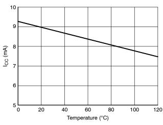
Figure 3. Supply Current vs. Temperature
