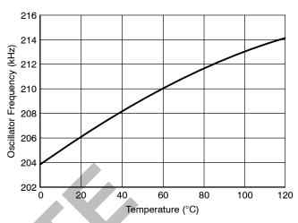
Figure 4. Oscillator Frequency vs. Temperature
