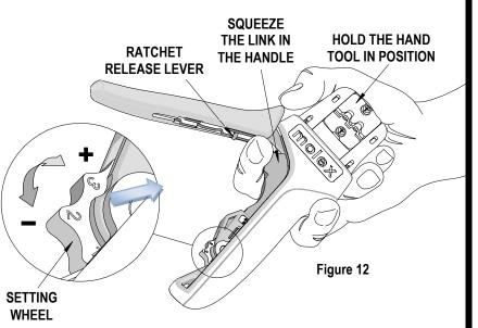
2. Rotate the setting wheel counter-clockwise (CCW) to increase handle force. The numbers will display higher. To decrease handle force rotate the setting wheel clockwise (CW).
