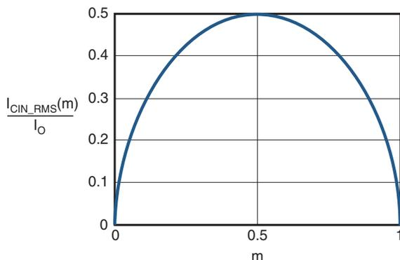
Figure 4. I<sub>CIN</sub> vs. Voltage Conversion Ratio
