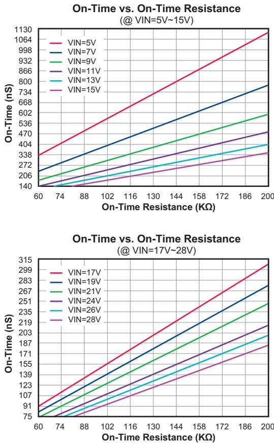
Figure 3. T<sub>ON</sub> vs R<sub>TON</sub> Curves for AOZ2261QI-11
