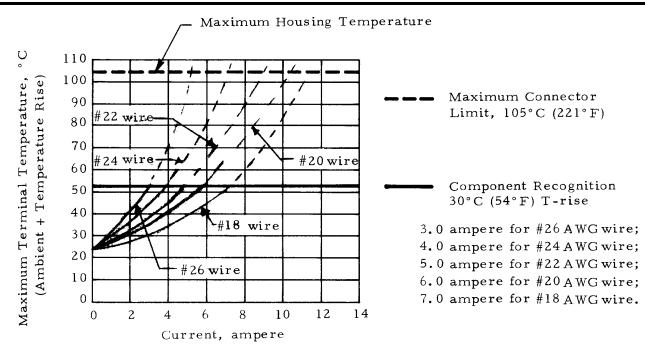
Figure 4 Terminal Temperature vs Current/Circuit 24 Circuit Assembly
