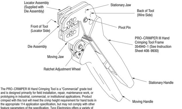
feature parameters of the specification. Tyco Electronics offers a variety of tools to satisfy your performance requirements. For additional information, contact the Tooling Assistance Center at 1–800–722–1111.
