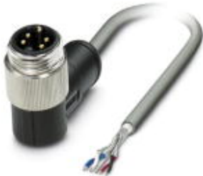
Bus system cable, DeviceNet, 5-position, PUR halogen-free, Gray RAL 7001, Plug angled 7/8"-16UNF, on Free cable end, Cable length: 20 m
