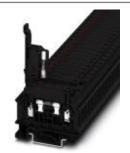
Fuse modular terminal block, Number of positions: 1, Connection method: Screw connection, Cross section: 0.2 mm<sup>2</sup>- 6 mm<sup>2</sup>, AWG: 24 - 10, Nominal current: 6.3 A, Nominal voltage: 500 V, Width: 8.2 mm, Fuse type: G / 5 x 20, Fuse type: Glass, Mounting type: NS 35/7,5, NS 35/15, NS 32, Color: black
