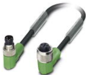
Sensor/actuator cable, 4-position, Variable cable type, Plug angled M8, on Socket angled M12, A-coded, cable length: Free input (0.2 ... 40.0 m)
