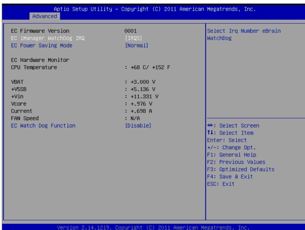
Figure 3.10 Embedded Controller Configuration
