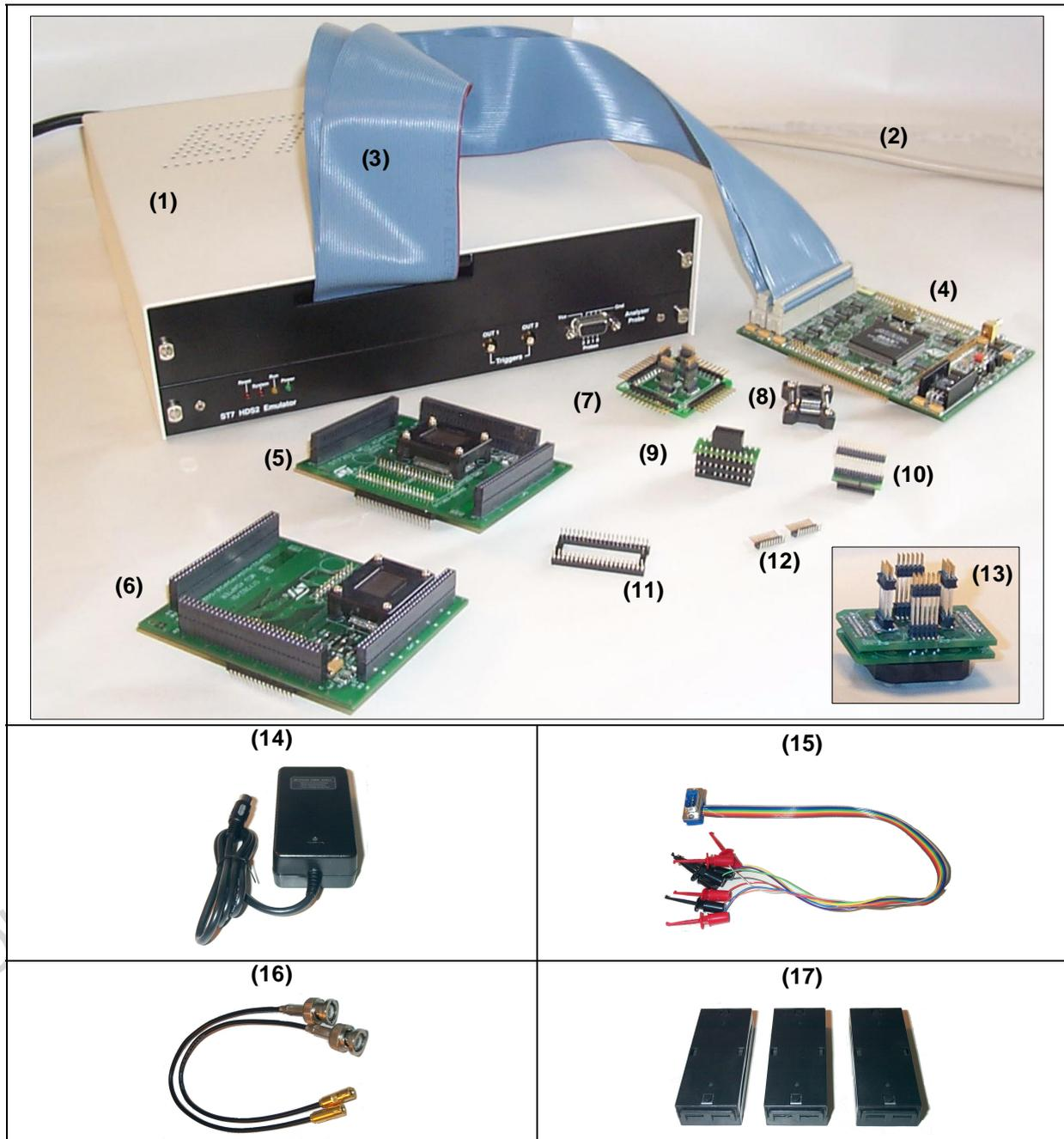
Figure 2: Main components of ST7MDTU2-EMU2B emulator kit
