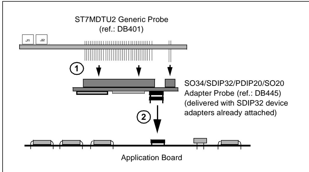
**Figure 15: SDIP32 MCU package connections**
