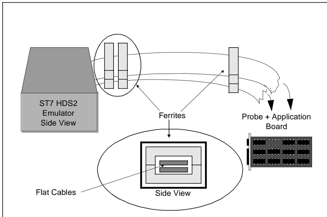
**Figure 6: Making your probes EMC-compliant**
