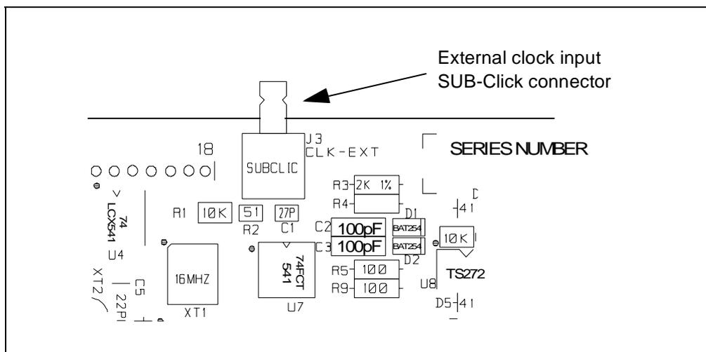
The SUB-click **external clock** connector on the probe can be used with the two SMB to BNC connectors provided in the emulator package. Voltage at these connectors must range between 0 V and 5 V. The levels are TTL.
