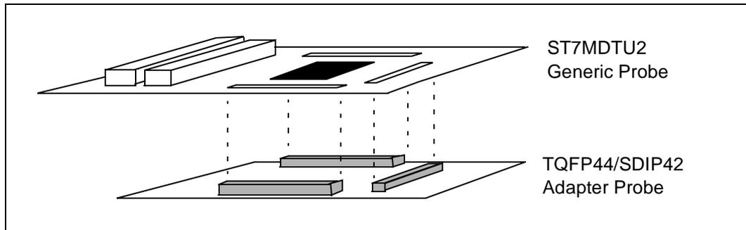
**Figure 8: Connecting the TQFP44/SDIP42 adapter probe to the ST7MDTU2 generic probe**
