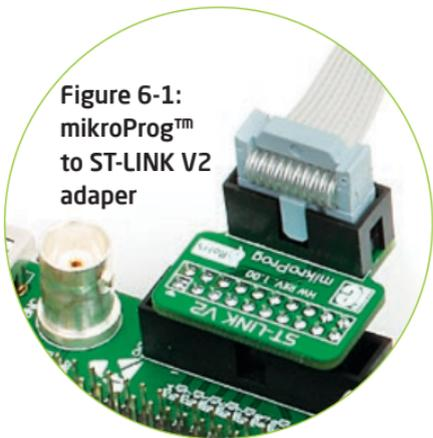
In order to connect mikroProg to 20-pin male JTAG connector it is necessary to use appropriate adapter, such as the **mikroProg™ to ST-LINK V2 adaper**, **Figure 6-1**. This adapter should be first placed on 2x10 male connector. Then you should plug in the mikroProg™ into 2x5 male header, **Figure 6-2**.
