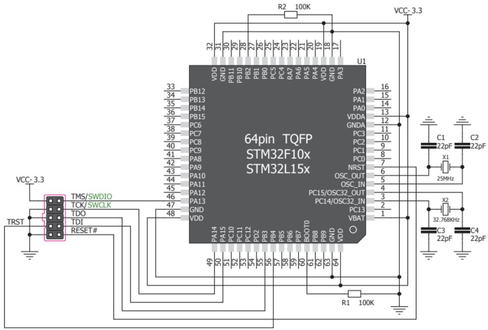
Figure 7-1: Connection schematics for 64-pin STM32F10x/STM32L15x MCU via 2x5 male header
