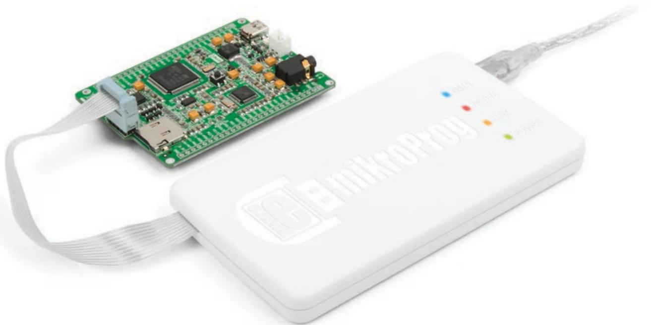
**mikroProg™ for STM32®** is a fast programmer and hardware debugger. Smart engineering allows mikroProg™ to support all STM32® ARM® Cortex™-M3 and Cortex™-M4 devices in a single programmer! Outstanding performance, easy operation, elegant design and low price are its top features. It is supported in mikroElektronika, as well as in other ARM® compilers.
