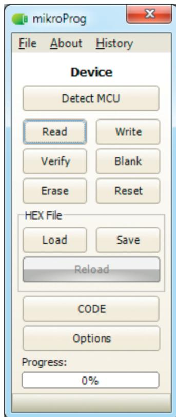
mikroProg™ for STM32® programmer requires special programming software called mikroProg Suite™ for ARM®. This software is used for programming all of STM32® ARM® Cortex™-M3 and Cortex™-M4 microcontroller families. It features intuitive interface and SingleClick™ programming technology. Software installation is available on following link:
