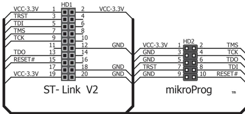
Figure 6-3: mikroProg™ to ST-Link V2 adapter connection schematics
