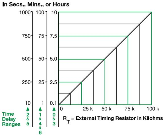
This chart applies to externally adjustable part numbers. The time delay is adjustable over the time delay range selected by varying the resistance across the R<sub>T</sub> terminals; as the resistance increases the time delay increases. When selecting an external R<sub>T</sub>, add the tolerances of the timer and the R<sub>T</sub> for the full time range adjustment.
