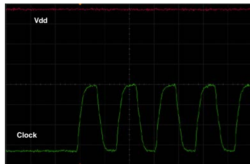
Figure 17. Startup Waveform vs. Vdd (Zoomed-in View of Figure 16)
