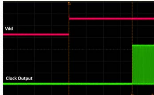
Figure 16. Startup Waveform vs. Vdd
